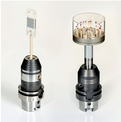
CT inspection items in accordance with VDE/VDI 2630
