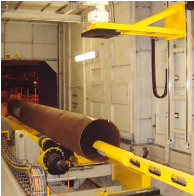
1 "Tube inside pipe" principle at a 21" pipe mill 2 Ceiling-mounted movable tube and high-voltage generator 3 Flat-panel detector in position close to tower 4 Flat-panel detector at end of boom
