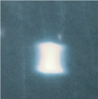
1 mm focal spot of a conventional MXR-160/20. At 640 W (maximum power) the temperature reaches 1500 °C.
