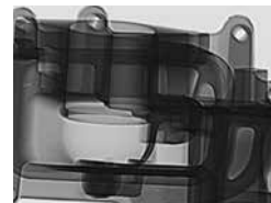
Al cast part with 95% HDR
