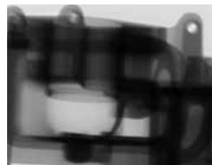
Al cast part with 15% HDR
